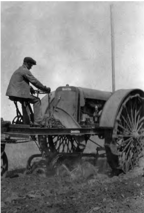
Square turn tractor, 1910, Carl driving. According to the manual, it turned a square corner in the field in 5 seconds. Built in Norfolk, Nebraska
