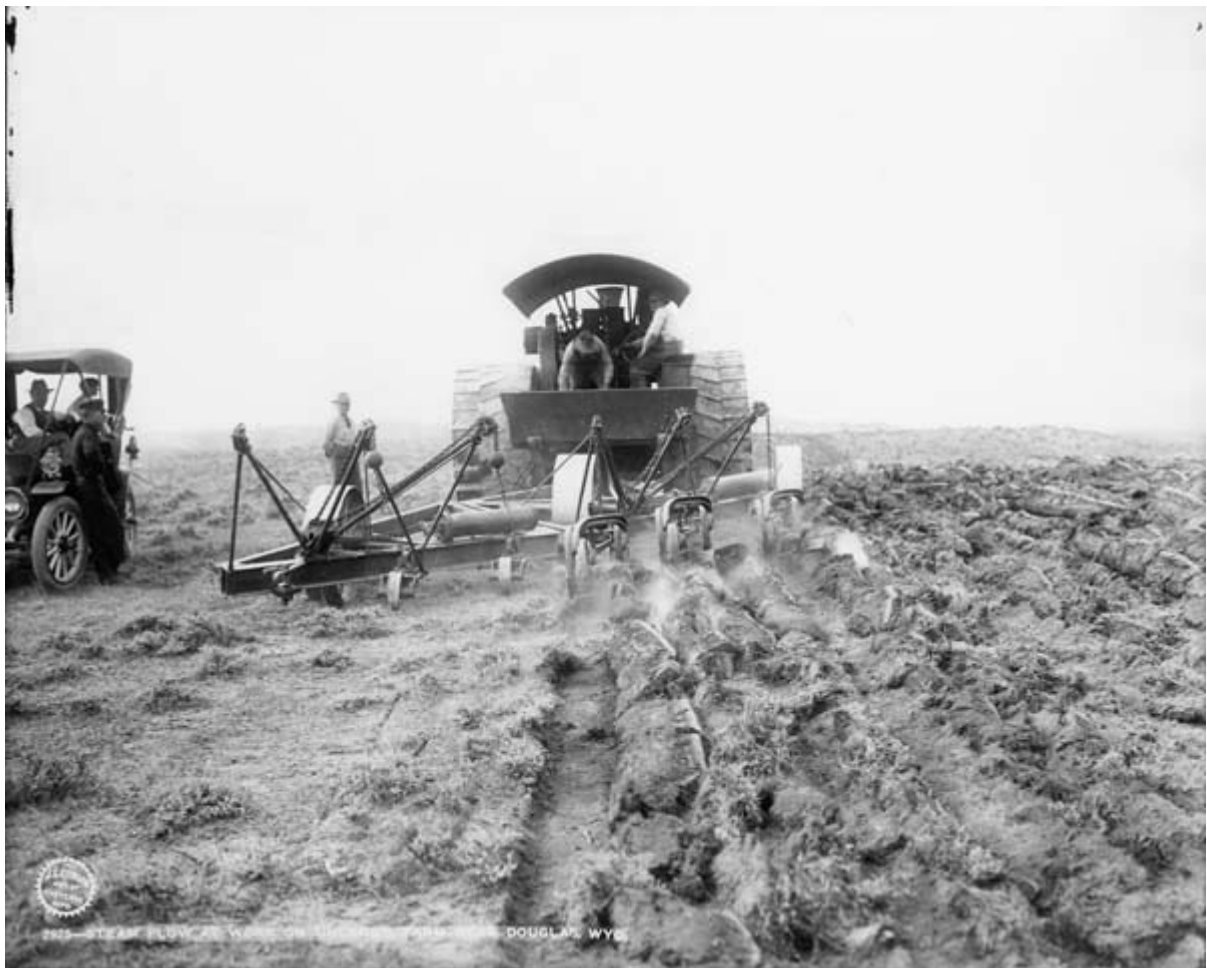
Steam plow on Unland's farm, Douglas. This steam tractor is breaking sod with a moldboard plow. Note the two operators on the tractor and the size of the machine. Photo: J. E. Stimson Collection, Wyoming State Archives, negative 2925.
